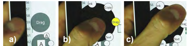
Figure 13: Pen Tools Widget: The mode is indicated when not in use (a). The marking menu appears on thumbpress (b), and changes mode when the thumb slides to a new tool (c).
