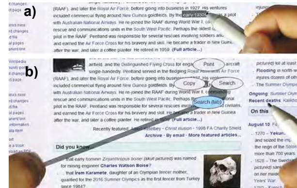
Figure 22: After selecting text with the pen (a), thumb input indirectly controls a context marking menu (b).
