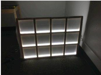
Figure 1: Prototype screen using visual light along the bottom of each grid square. While functional as an input mechanism, the prototype does not allow for simultaneous rear projection.
