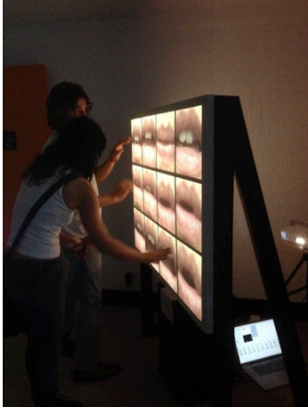
Figure 2: Two people interacting with the spandex fabric grid interface, and the projector and computer system behind the screen.
