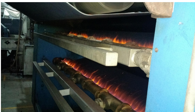
Figure 3. Singeing, i.e. burning with open flames, is a standard procedure that textiles are subjected to after weaving.
