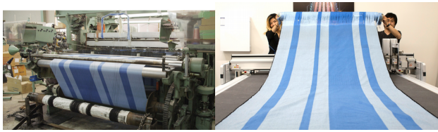
Figure 10. Left: Weaving interactive Jacquard textile Right: Interactive areas are in various locations
