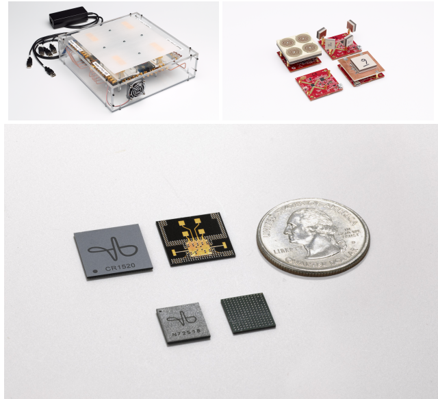
Figure 9: Top: Early prototypes of Soli FMCW and impulse radars. Bottom: Soli radar 60 GHz chips with antennas-in-package (AiP).
