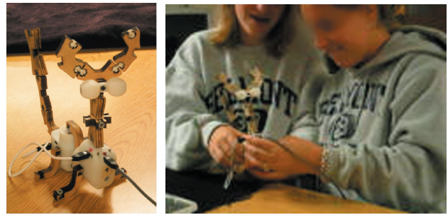
Figure 6. One 8 th grade group's “moose” walked with 2 DOF rotation. The group programmed it collaboratively.
