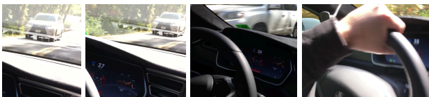
Image 1. Autopilot on, sun glare on camera Image 2. Autopilot alarm starts Image 3. Car veers suddenly left into lane of approaching car. Image 4. Driver grabs wheel and turns quickly right, “Whooo-a”
