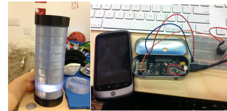
Figure 2. Costumes had embedded Android-based mobile phones connected to Adafruit mini IOIO boards that drove the light displays.
