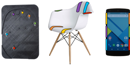
Figure 4. The three prototype configurations: Hand Pad , Chair , and Smartphone , and their electrode arrangements. Colors indicate the electrode connection position on the custom sensor board.
